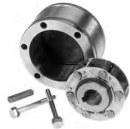
This **Backstop** option helps prevent reverse rotation in high stop-start loads, and results in less wear and longer life. Its centrifugal throw-out design eliminates sprag sliding and reduces wear. It operates with standard and EP lubricants and requires no external lubrication.
