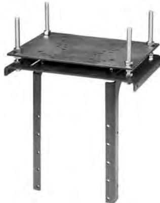
This **Modular Motor Mount** is attached and supported by two angle iron brackets with equally spaced holes, which align with the spacing of the cast slots of the gear case. This way, the motor mount can be adjusted up or down depending on the customer's requirements. It can also be mounted on the side of the reducer for screw conveyor applications.
