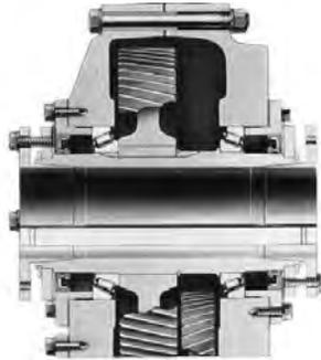
A tapered bore in both sides of the reducer's output hub snugs up against a matching taper on the outer surface of the bushing . . . "Twin Tapered".
