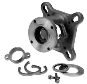
The screw conveyor drive shafts are made from high alloy steel and engineered to CEMA dimensions. They are three-bolt drilled and their tapered fit ensures simple installation. The rugged locking plate (patent pending) also provides a mechanical shaft removal feature. #316 Stainless Steel drive shafts also available.
