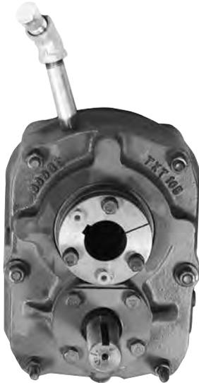
Dodge Torque-Arm Speed Reducer. The speed reducer shall be either a belt driven or direct coupled enclosed shaft mount type unit with a single or double reduction ratio. The reducer shall mount directly on the driven shaft and utilize an adjustable Torque-Arm that attaches from the gear case to the support structure or foundation.
