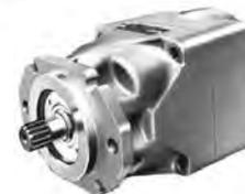
**Hydroil Vane Motors** are superior single stage vane type fluid motor. A series of internal ports admit oil to and carry it from the power element. Complete hydraulic balance of the assembly contributes to the mechanical efficiency and long life of these motors as well as to their unusually quiet operation. Other exclusive features assure a minimum of friction and efficient valving action regardless of operating speeds.
